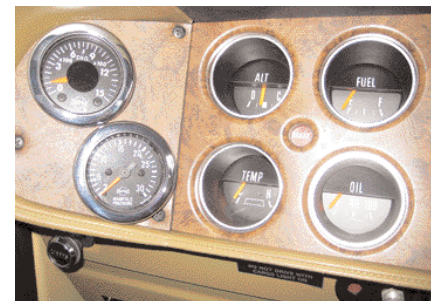
The instrument panel is classic Dodge, except for the addition of pyrometer and manifold pressure gauges.
